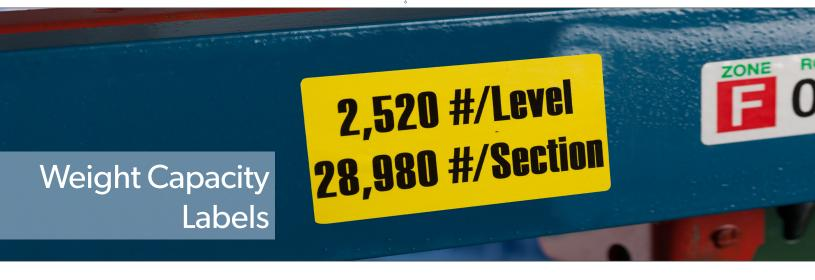
**Weight Capacity Labels** increase warehouse safety by ensuring workers and forklift operators are loading the racks properly. By not having labels properly displayed, the racks could be overloaded and cause a failure. Be sure to comply with your rack manufacturer for capacity ratings.
